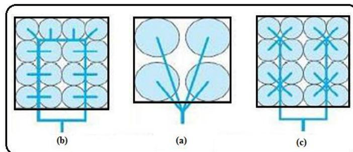
**Figure 3:** Collection devices of biogas [12]. (a) Each well is connected to an extraction installation by a separate pipe; (b) The wells are connected to a ring line; (c) The wells are connected to each other and then to the extraction unit: used when there are a large number of wells.
