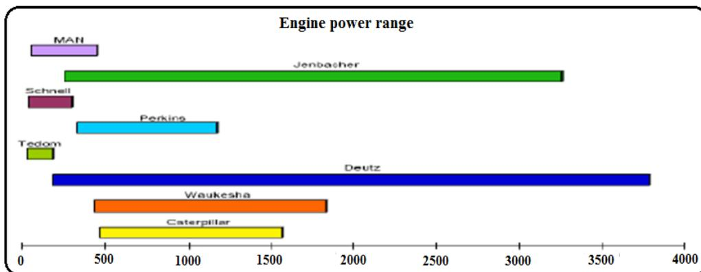
**Figure 1:** power range of different brands of biogas engines [8].
