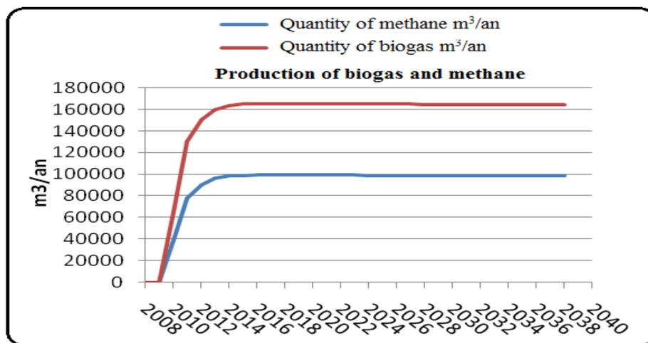
**Figure 4:** Results of estimating biogas production by years
